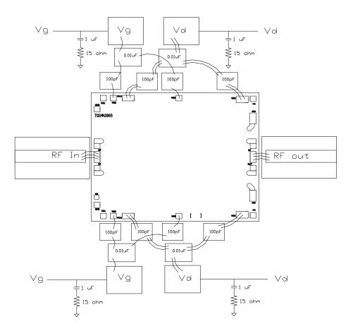
GaAs MMIC devices are susceptible to damage from Electrostatic Discharge. Proper precautions should be observed during handling, assembly and test.
